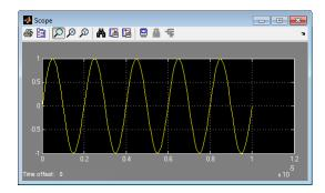
The Sinusoid specifies a 1-V amplitude for the modulation on  $f_{RF}$ , which the mixer downconverts to  $f_{IF}$ . The SimRF Outport block probes the intermediate frequency and recovers the 1-V modulation amplitude. This value agrees with a specified conversion gain of 0 dB in the mixer.
