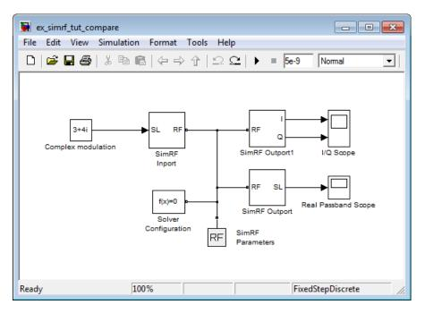
The system simulates a real passband signal as the real part of a complex passband signal according to the formula
