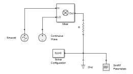
This configuration specifies an AM waveform at the input port of the mixer, an LO at the LO port of the mixer, and a  $50-\Omega$  termination at the output of the mixer.
