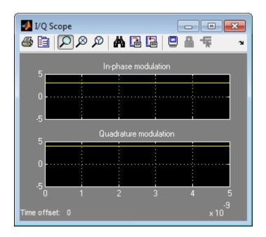
The 1-GHz carrier itself does not appear in the output. The results correspond to the real and imaginary parts of the Complex modulation at the input of the system. They also correspond to the In-phase modulation and Quadrature modulation blocks in "Simulate a Passband Signal in Simulink Software" on page 1-4.
