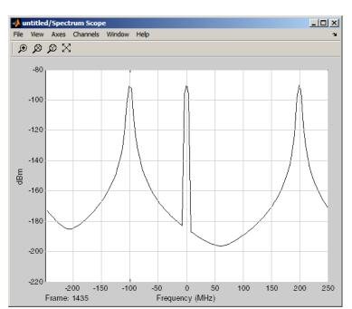
The following plot shows the RF filter input signal you specified in the Sine Wave block.
