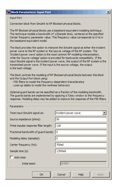
**Note** You must enter the **Sample time** (s) because the Input Port block does not inherit a sample time from the input signal. The specified sample time must match the sample time of the input signal. The Sample time (s) of 1/500e6 second used in this example is equivalent to a bandwidth of 500 MHz.
