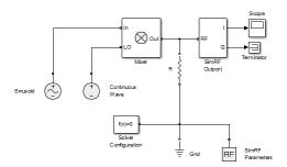
This configuration uses a SimRF Outport block as a voltage sensor at the output port of the mixer. The Simulink signal at the outport is the envelope of the carrier or carriers specified in the block. A scope attached to the outport plots the envelope. The **Output** parameter controls how signals are presented at the output ports. To change the appearance of the block, follow one of the workflows in the "Specify Block Parameters for RF Simulation" on page 2-11 section of this tutorial.
