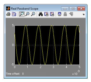
The output signal at the Real Passband Scope has a magnitude of 5 and a phase shift of atan2d(3,-4), or about 143°.
