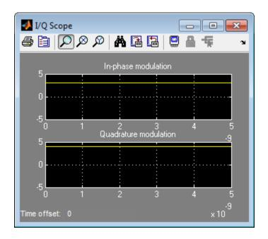
The I/Q Scope displays the in-phase and quadrature baseband components of the 1-GHz signal. The 1-GHz carrier itself does not appear in the output. The results correspond to the real and imaginary parts of the Complex modulation at the input of the system.
