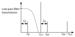
The preceding figure illustrates low-pass filtering of a low-side injection system. Mixing  $f_{RF}$  and  $f_{LO}$  produces signals on the carriers  $f_{IF} = f_{RF} - f_{LO}$  and  $f_{RF} + f_{LO}$ . Adding a low-pass filter to the model reduces the power present in the high-frequency signal.
