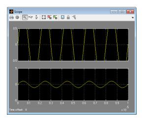
The first set of axes displays the modulation of specified carrier  $f_{IF} = f_{RF} - f_{LO}$ . This carrier appears on the first set of axes because the **Carrier frequencies** parameter of the outport specifies it first. The second set of axes displays the modulation at  $f_{RF} + f_{LO}$ . The modulation of the upper mixing product has the same amplitude as the modulation of the downconverted signal.
