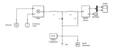
This configuration models a third-order low-pass Butterworth filter with a cutoff frequency of 1 rad/ns, or about 0.159 GHz. The high-frequency mixing product is in the stopband of the filter. The low-frequency product is in the passband.
